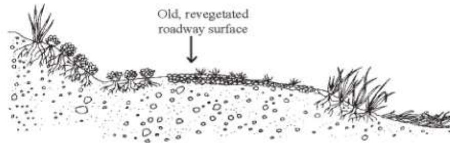
c. Decommissioning - Permanent Road Closure with Surface Scarification and Seeding for Revegetation, but Keeping Most of Road Template (Shape).
